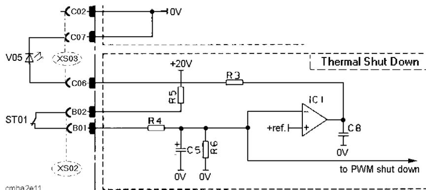
This circuit interrupts the gate pulses from the pulse width modulator if the machine is overloaded. When it has not operated due to high temperature, the thermal overload cutout normally short-circuits inputs B01 and B02. If the cutout contact opens, IC1 lights LED V05 and the pulse width modulator (8) blocks the gate pulses. See also ST01 in the component description.
