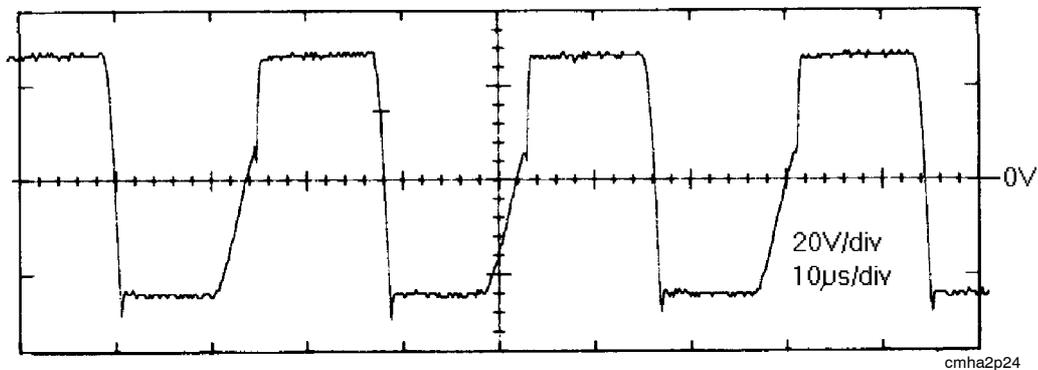
*Primary voltage at TC02 for 30 V across the buffer capacitor*
