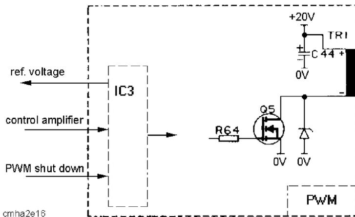
The pulse width modulator determines the frequency and pulse time of the control pulses to the MOSFET transistors.
