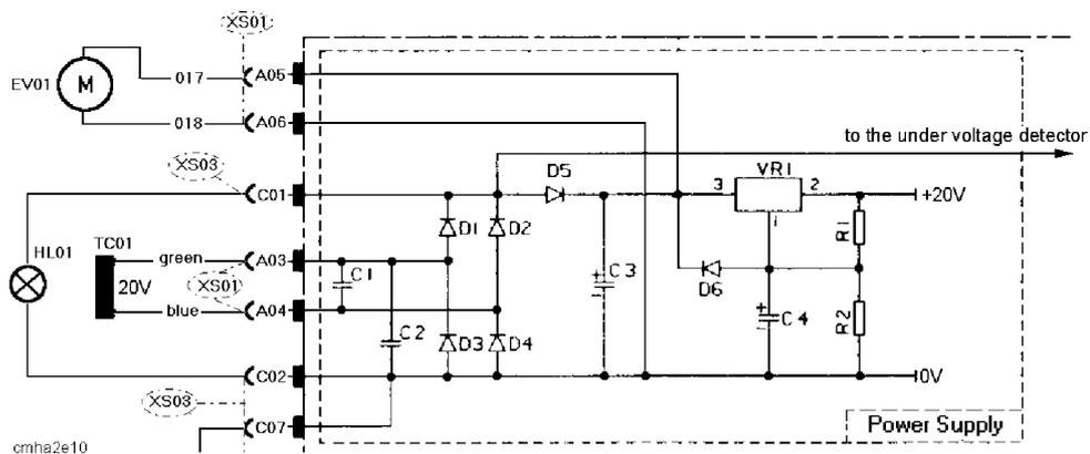
Rectifier bridge D1-D4 is supplied at 20.5 V from transformer TC01. The rectified voltage is stabilised by voltage regulator VR1 to  $+20 \pm 1$  V. All circuits on the circuit board except the current reference (6) and the gate circuit (9) are supplied from VR1.
