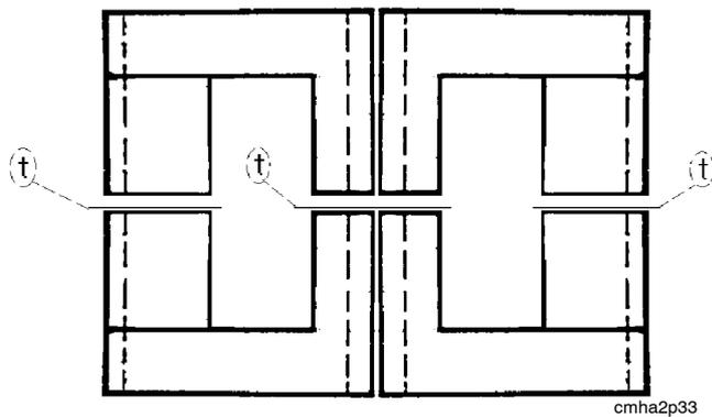
*Airgap (t) in the transformer core*
