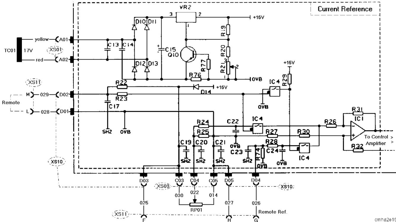
This circuit supplies a signal voltage to the current setting potentiometer and remote control unit. It also modifies the current reference signal to a suitable level for the control amplifier (7).
