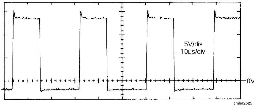
*Gate pulses as measured across the dummy gate load on circuit board AP01 between connections F01 and F02.*
