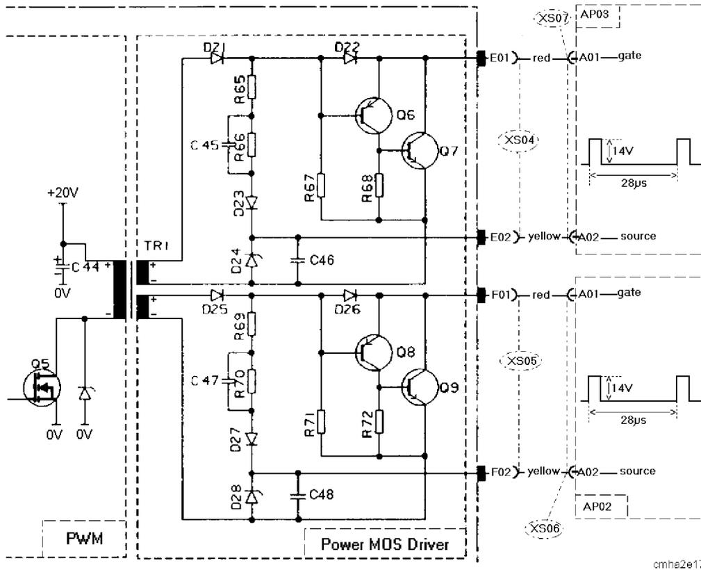
The driver stage for the MOSFET transistors provides control pulses to the gate-source of the power transistors. There is a separate output for each switching unit.
