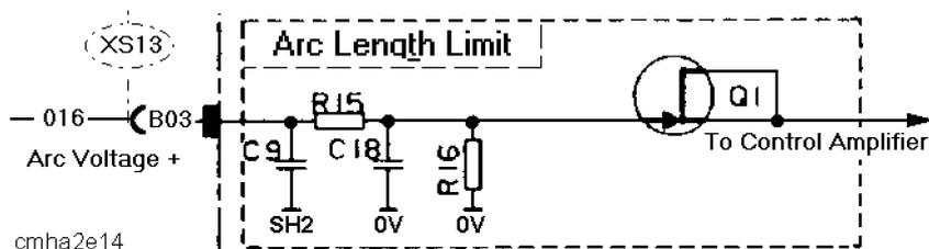
This circuit, which restrict the arc voltage and open-circuit voltage, assists in limiting the arc length when welding in the 20 - 50 A current range.
