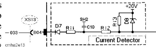
This voltage is rectified and smoothed by D7, R11 and C10, to provide a voltage after R11 of +3 to +3.5 V at no-load and -10 to -50 V when welding. This signal interrupts the Hot Start (starting current boost), the length (200 ms) of which is controlled by the control amplifier (7).
