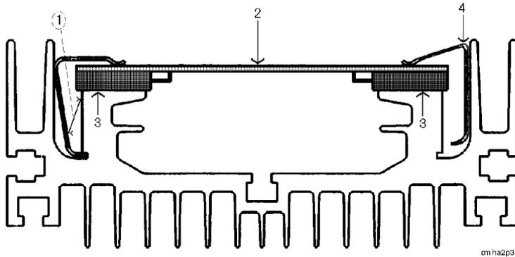
Removal/refitting of transistor circuit board
